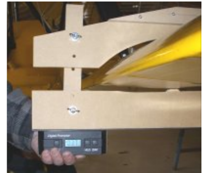
An inclinometer is used on the rigging board to get the correct angles.
