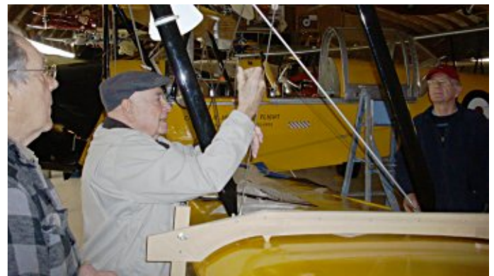
Twisting and turning – the tension on the wires is adjusted by Bill Orbeck, with Ray Fessenden assisting.
