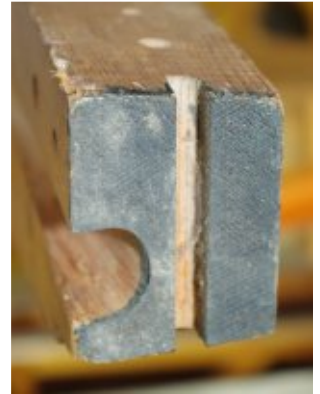
An original wing spar as made by de Havilland.
