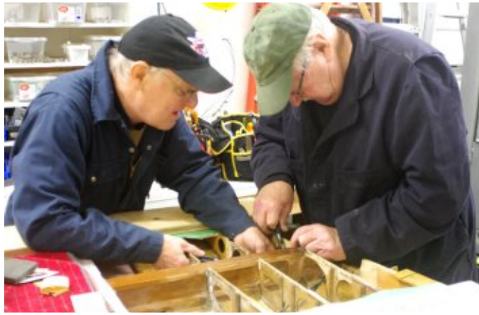
Peter Roberts and Cyril Meadows add stiffness and support to the ribs in the wingwalk area.
